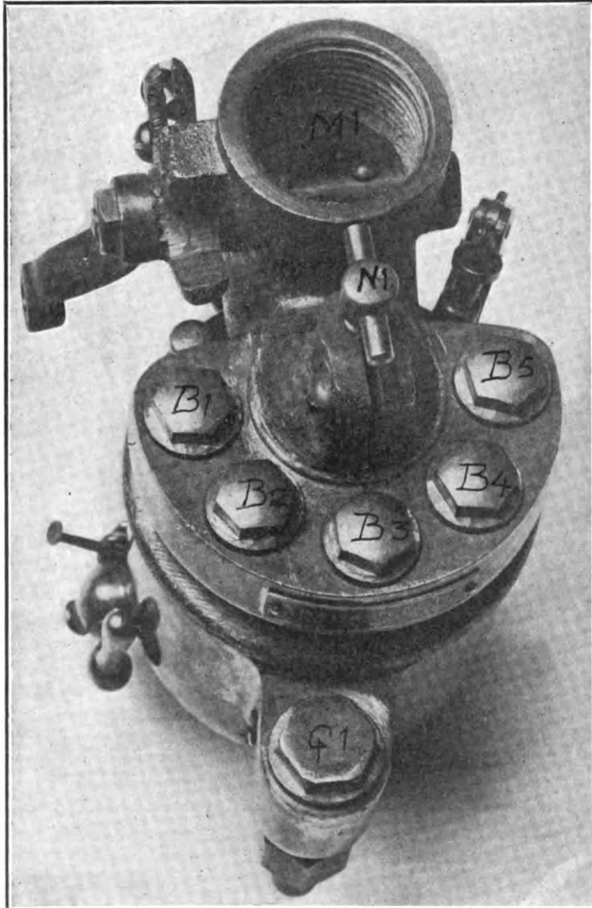
Fig. 8—Looking down upon the carbureter, showing the orifice for connecting the intake manifold and the caps covering the floating balls
